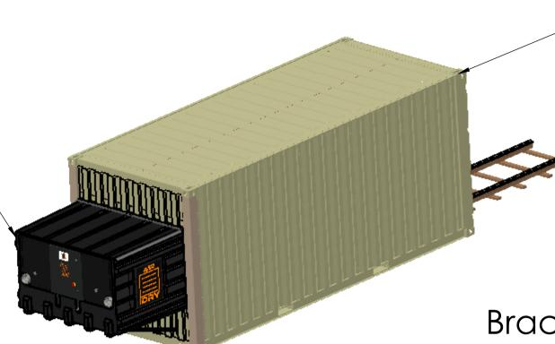
Bracket Spacing Must Match Ribs on AIR Module See Container Endwall Detail for Height
